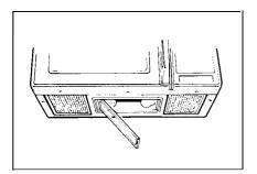
Be sure bulbs to be replaced are cool before removing. Break the adhesive seal by gently unscrewing the bulbs. Replace with 40-watt incandescent bulbs (WB02X4253) available from your GE supplier. High intensity 40-watt bulbs (40S11N/1), which are available in supermarkets and hardware stores, may also be used for replacements. Raise light compartment cover and replace screw. Connect electrical power to microwave oven.
